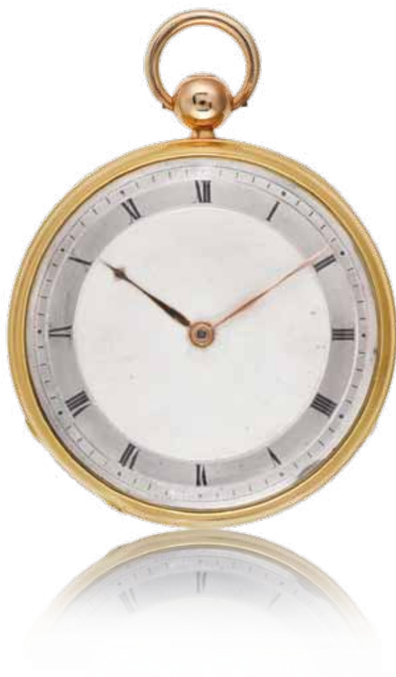
Vacheron Constantin, Pocket Watch, grande and petite sonneries, quarter-repeater Geneva (Switzerland), 1827 18K pink gold, silver dial Caliber 22", quarter-repeater, round, in gilt brass, cylinder escapement, three-arm annular balance, flat balance-spring, simple adjustment index, 4 holes with jewels, key winding and setting diam. 6.4 cm Vacheron Constantin Heritage Collection N° 10715
